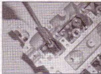
9.5 Push the oil seal into position using a suitable tube or socket
