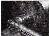
7.16a Tighten the hub nut to the specified torque setting while rotating the drum
