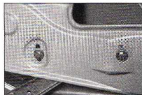
14.14a Mark the position of the regulator guide bolts on the door, then undo the bolts ...
