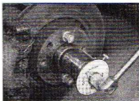
2.18b . . . and then through the specified angle (note the use of an angle gauge)
