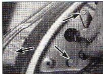
19.5 Disconnect the wiring connector, then undo the three retaining bolts (arrowed) ...
