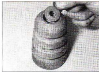
14.24a When refitting the bump stop, do not omit the washer from inside the stop ...
