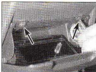
28.6b ... then open up the ashtray, and undo the two upper retaining screws
