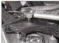
4.7 Tighten the strut upper mounting nuts to the specified torque setting
