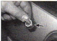
18.2c ... and lift off the washer and outer mounting rubber (arrowed)
