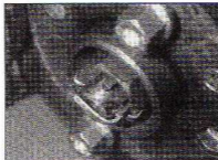
2.19b . . . and secure in position by bending over the split pin ends
