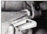
14.3 If the right-hand spring is being removed, also remove the brake pressure-regulating valve spring clamp
