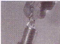
34.10 Adjusting a spark plug electrode gap using a special tool
