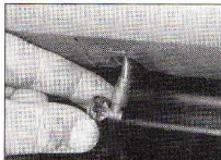
15.5b ... and disconnect it from the hose (1.6 litre DOHC model – jet mounted in spoiler)
