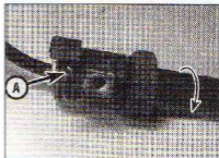
20.30 Turn the sensor in the direction of the arrow, so that the retaining clip (A) is freed from the mounting bracket
