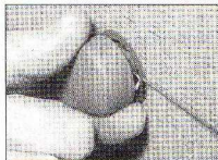
12.6 On models with manual windows, unhook the regulator handle retaining clip using a piece of welding rod
