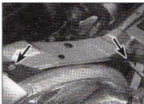
7.2b ... then undo the two headlight unit retaining bolts (arrowed)
