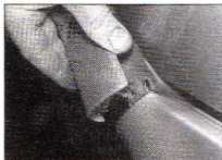
7.3a Release the end of the bumper from the wheelarch outer trim cover ...
