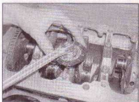
18.20d ... then through the specified Stage 2 angle using an angle tightening gauge
