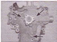
7.7 Coolant pump short retaining bolt locations (arrowed) – 1.0 and 1.2 litre DOHC engines (shown with timing cover removed)
