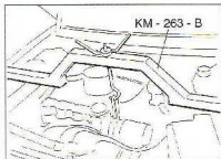
8.9 Vauxhall/Opel tool No KM-263-B used to support engine
