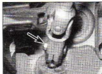
20.3b . . . and the intermediate shaft-to-steering gear clamp bolt and nut (arrowed)
