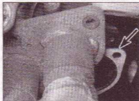
17.10b Use a new gasket (arrowed) when reconnecting the exhaust front section to the manifold – DOHC engine
