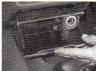
6.17 Withdraw the ashtray unit from the fascia ...
