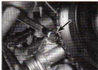
6.27 Unbolt the crankshaft speed/position sensor bracket from the oil pump. Securing bolt arrowed – 1.4 and 1.6 litre DOHC engines
