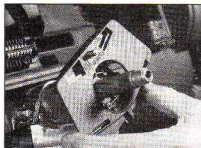
28.10b ... then turn the combination switch mounting bracket anti-clockwise, and slide it off the steering column
