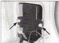
17.3 ... to gain access to the central locking control unit (retaining bolts arrowed)
