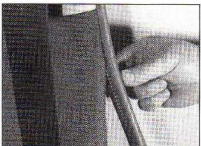
25.10a ... then peel the door sealing strip away from the front of the panel ...
