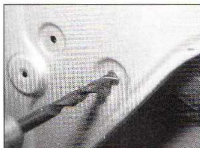
14.15b Carefully drill out the rivets with a suitable drill ...
