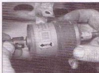
21.9 Ensure that the flow direction arrow points in the direction of fuel flow
