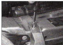
7.2a Undo the bolts securing the radiator grille section of the front bumper to the crossmember ...
