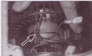
9.59 Secure the blower motor in position with the retaining clip, making sure its wiring is correctly routed through the clip (arrowed)
