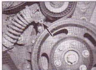
5.6a Lever the drivebelt tensioner roller clockwise, until the hole in the tensioner arm (arrowed) is aligned with the corresponding hole in the tensioner body – 1.2 litre DOHC engine
