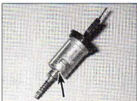
18.7 Later type of lock cylinder. Early types have a hook cast onto the end of the lock cylinder in the position indicated by the arrow
