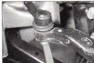
21.4 Unscrew the retaining nuts securing each track rod balljoint to the swivel hubs
