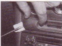
9.4b ... then carefully prise out the lever surround. Note the use of a piece of card to avoid marking the fascia panel
