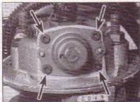
12.39a Unscrew the fuel pressure regulator securing screws (arrowed) ...
