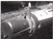
23.2b . . . and insert it into the slot, making sure that it is correctly engaged with the tensioner pin (arrowed)
