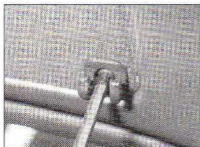
15.2 Undo the retaining screws, and remove the parcel shelf lifter hooks from the tailgate ...
