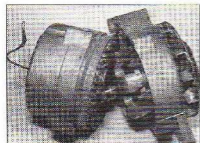
7.23 Separating the drive end housing from the slip ring end housing – standard Delco-Remy alternator
