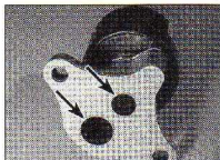
5.15 Check the exhaust gas recirculation valve vent holes (arrowed) for contamination - X 12 SZ and X 14 SZ engines
