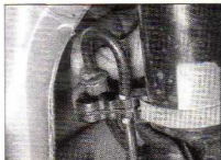
4.2 On models with ABS, free the sensor wiring from its clip on the base of the strut
