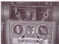
9.5a Undo the four retaining screws (arrowed) ...
