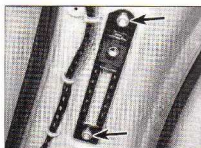
25.21 Rear seat belt height adjuster mechanism is retained by two bolts (arrowed)
