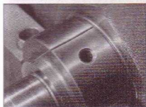
18.7 Lay the length of Plastigauge on the journal to be measured, parallel to the crankshaft centre-line
