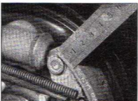
5.3a Brake shoe wear can be assessed by measuring the thickness of the friction material . . .
