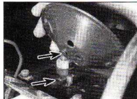
14.20 Fit the bump stop seat, making sure its locating peg is engaged with the inner retaining plate hole (arrowed)
