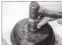
10.9b ... and drift it into position using a hammer and tubular drift
