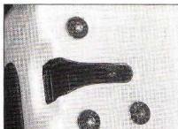
13.25b ... then undo the three lock retaining screws ...
