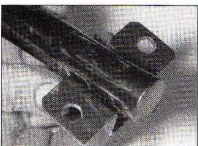
8.8 When refitting, ensure that each lower clamp is correctly engaged with the anti-roll bar flats
