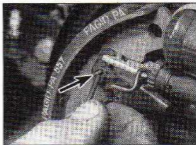
5.7 Remove the retaining spring, followed by the lever and return spring (arrowed)
