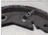
5.17 It may be necessary to transfer the adjusting lever pivot pin and clip (arrowed) from the original shoes to the new ones
