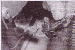
11.22 Disconnecting the wiring plug from the coolant temperature sensor – engines with multi-point fuel injection
