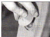
25.6a Prise out the circular plug (where fitted) from the front of the luggage compartment side trim panel
