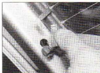
15.4b ... and the heated rear window wiring connector ...
