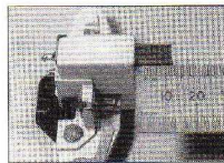
7.5 Measuring the length of an alternator brush - standard Bosch alternator
