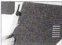
13.23b ... and remove the trim panel to gain access to the lock
