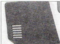
17.11b ... and remove the trim panel to improve access to the servo unit
