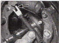
5.24 Refit the adjuster strut, noting that the longer, straight part of the fork (arrowed) must be behind the shoe
