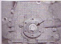
6.19 Slacken the crankshaft pulley hub retaining bolt (arrowed)
