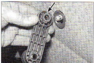
12.15 When refitting, fit the clip (arrowed) to the regulator handle before fitting the handle to the door
