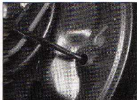
7.7a If necessary, release the handbrake lever stop-peg by inserting a screwdriver lever through the hole in the rear of the backplate ...
