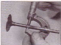
8.10 Measuring a valve stem diameter
