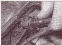
15.46b ... and the brake servo vacuum hose from the upper section of the inlet manifold
