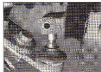
2.5 Withdraw the clamp bolt, and free the lower arm balljoint from the swivel hub
