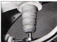
14.10 Unscrew the retaining bolt from the centre of the bump stop, and remove the stop from the vehicle
