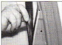
13.16 Free the sealing strip from the rear of the door to gain access to the guide upper retaining bolt
