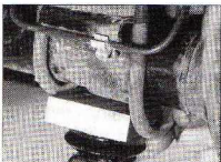
14.7a Undo the retaining nuts, then withdraw both U-bolts ...
