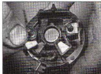
10.18b ... and recover the insulator plates - Valeo starter motor
