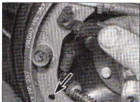
5.25 Refit the adjusting lever and spring, making sure that the spring is correctly engaged in the front brake shoe hole (arrowed)
