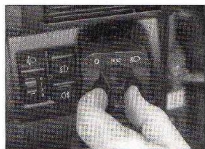
4.8 Depress the retaining clips, and withdraw the lighting switch from the fascia
