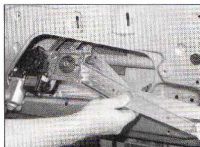
14.15d ... and remove the regulator assembly from the door
