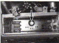
28.13a Undo the retaining screw (arrowed), then slide out the radio/cassette bracket, freeing the wiring connector ...
