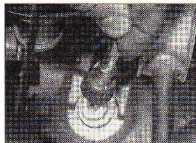
5.1 Disconnecting the speedometer cable from the gearbox
