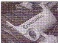
34.18a Removing the plastic cover from the camshaft cover - 1.4 and 1.6 litre DOHC engines
