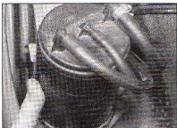
4.8 Note the locations of the charcoal canister hoses
