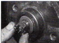
7.4a Slacken and remove the hub nut and washer ...
