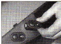
4.31 . . . then release the retaining clips, and slide the relevant switch out of the pocket
