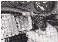
19.5 Depress the retaining clips, and slide the combination switches out from the column ...
