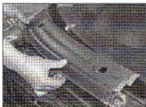
17.3 Removing the right-hand windscreen cowl panel
