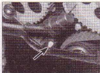
6.9a Lower outer timing belt cover upper securing bolt (arrowed) . . .
