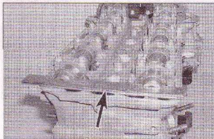
10.57 Before refitting the cylinder head, insert the camshaft setting tool (arrowed) into the slots in the ends of the camshafts
