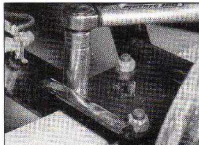
14.19 Tighten the U-bolt retaining nuts to the specified torque as described in text
