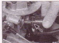
12.45b ... and withdraw the idle speed control motor. Note O-ring (arrowed)
