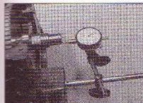
11.5 Check the crankshaft endfloat using a dial gauge...
