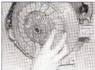
4.10 Place the friction disc on the flywheel, with the greater-projecting side of the hub facing away from the flywheel
