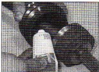
3.16 Pack the CV joint and gaiter with the grease supplied
