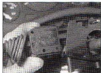
4.3a Depress the retaining clips, then slide out the switch (shown with steering wheel removed for clarity) . . .
