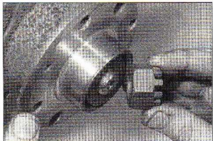
2.11 Engage the swivel hub with the driveshaft constant velocity joint, and fit the washer and new retaining nut
