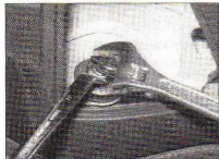
12.4 Slacken the mounting nut whilst retaining the piston with an open-ended spanner
