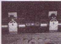
10.3b Camshaft bearing cap numbers (exhaust camshaft shown)
