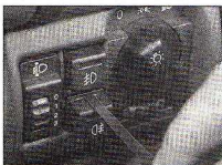
4.12 Using the hooked tool to withdraw the front foglight switch
