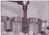
11.39b Tighten the cylinder head bolts to the specified torque ...
