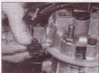
12.10 Sliding the fuel injector wiring rubber grommet from the fuel injection unit
