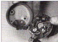
10.17 Removing the rear cover - Valeo starter motor
