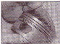
17.10 Fitting an oil control spreader ring
