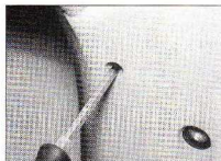
25.20b ... then undo the upper retaining screw ...
