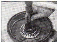
10.5 Support the hub on blocks of wood, and drift out the outer races using a hammer and punch
