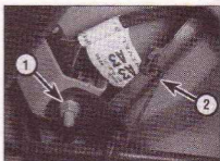
6.17 Fuel tank strap securing nut (1) and handbrake cable bracket (2)
