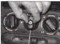
4.18 Release the retaining clip with a suitable screwdriver, and pull off the knob
