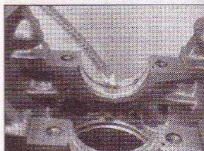
18.16 Lubricate the main bearing shells before fitting the crankshaft
